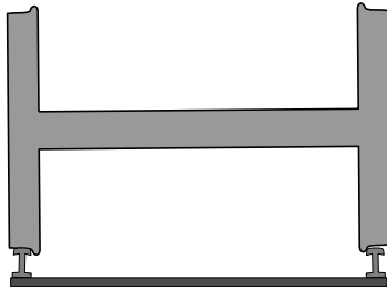
Fig. 3. Wheelset on rails. The evolving surfaces result in complicated relations between lateral shift, elevation and contact point position. For an elastic axle, such relations (dependent on yaw and, in general, also on revolution angle) hold for each of the wheels. For a rigid wheelset, also the rolling angle is determined by a holomorphic constraint
